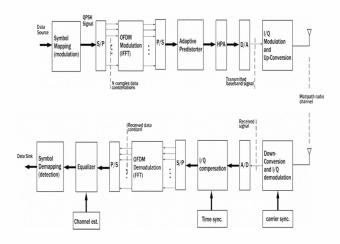
Figure 1 The CP-free ST-BC MIMO-OFDM systems under HPA and IQ-imbalance.
