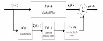
Figure 3 Block diagram of GSC-based equalize with PA.
