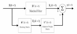
Figure 2 Block diagram of the GSC-based equalizer.
