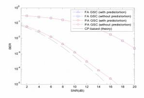
Figure 4 Performance comparisons of the CP-free ST-BC MIMO-OFDM system with and without adaptive predistorter.
